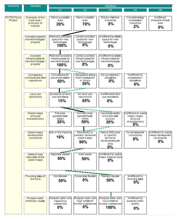
Figure 3. Pumped hydroelectric storage (PHS) at former open pit coal mines.
